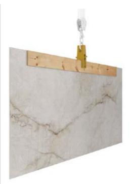
If a double **clamp** is not available, a **single** one can be used, enlarging its contact point by inserting a strip of wood of 300x20x2 cm. This is necessary to rotation or twisting of the slab, which could cause it to break.
