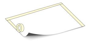
Secure the corrugated cardboard with adhesive tape around the edges so that no sand or other material can get underneath the protective layer during the construction works. It is essential not to allow sand or dust to get underneath this protective layer.
